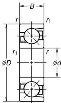
**Bearing Nomenclature (HPS Angular Contact Ball Bearing)**
