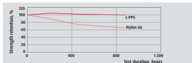
Heat resistance | Heat resistance at 180 °C
