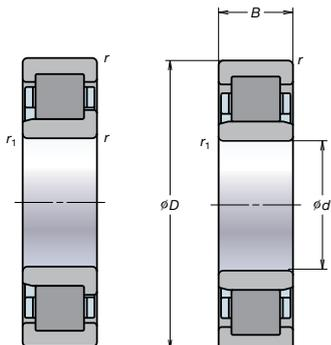
**Bearing Nomenclature (High Load Capacity Cylindrical Roller Bearings)**
