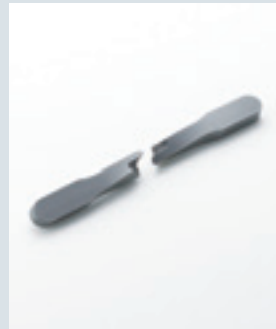
Torsion evaluation with a density of 6.8 g/cm 3
