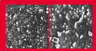
Distribution and size of carbide and carbonitride particles in Super-TF material (left) compared to distributionand size in a standard material (magnified by 4.000).
