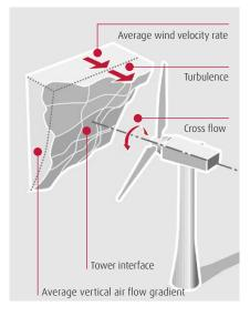
Air Flow Profile of a Wind Generator Plant Partial wind velocity depends on rate, place and time and results in considerable dynamic load impacts affecting the plant as well as subassemblies including the rolling bearings.
