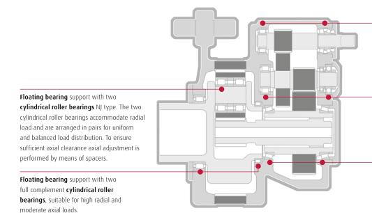
Combination of thrust bearing and floating bearing arrangement with a **cylindrical roller bearing** and a **tapered roller bearing** arranged in asymmetric pairs, suitable for high radial loads and high axial loads from one direction.
